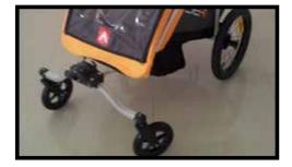
To remove the swivel wheel, simply push the red button on the rear of the connecting block, and pull the wheel out.
