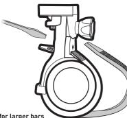
NOTE: Remove the inside bushing for larger bars
